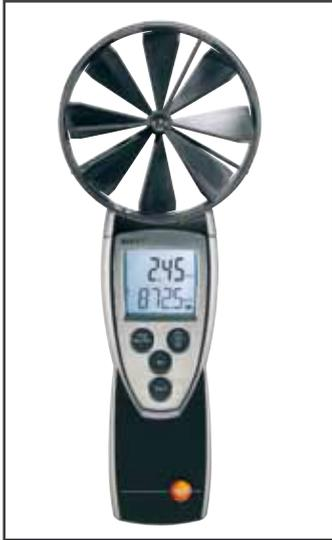
Propeller-type flow meter,
