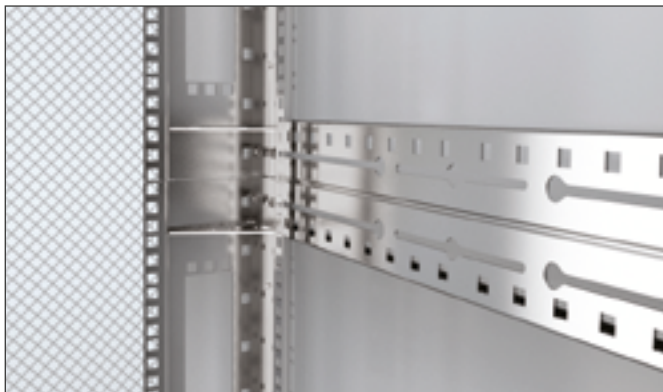
Rear pair of 19" extrusions is vertically divided to allow for various depth settings to accommodate different servers.
