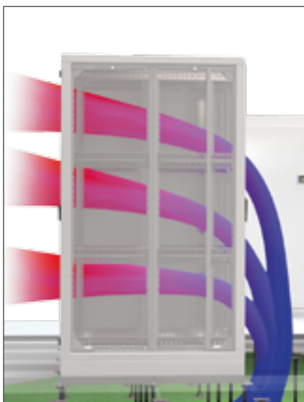
Cold air is delivered to the cold aisle using a raised floor as a cold air handling plenum. The hot air is blown out on the back side to the hot aisle.
