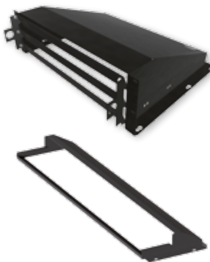
An air flow deflector is used to direct the cold air (which is coming from raised floor plenum) to the front part of rack. A louvre can be used to stop the air intake if no equipment is installed.
