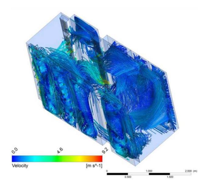
Picture shows general view on streamlines within the confined cold aisle.
