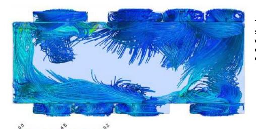
The picture shows air streams within the confined aisle for cooling units with difusors.
