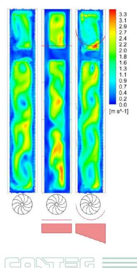
The specially designed air separation plates with deeper semi-rounded V-shape resulted, as expected, into a stable the air-flow rejected from the cooling unit. The goal of use of separators was to eliminate interaction between multiple air streams.
