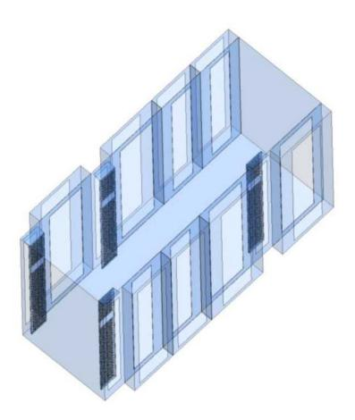
The mathematical model of the contained cold aisle, which was created and investigated to confirm measured data, is shown on the 3D picture.
